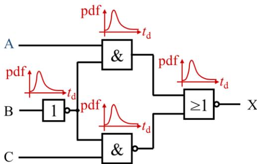
**Figure 1: Combinatorial block with variable delay**
