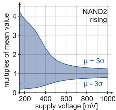
**Figure 2: Normalized  $3\sigma$  values of gate delay at various supply voltages**
