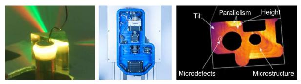
Left: Whispering-gallery based laser, Center: Holography system for industrial applications, Right: Holographical analysis of a practical component
