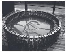
A 1.6 m diameter water-filled wave tank with 50 actuators generating an "S" using dynamic surface waves, designed and fabricated at Osaka University in Japan. Your job: make it 320 times smaller.
