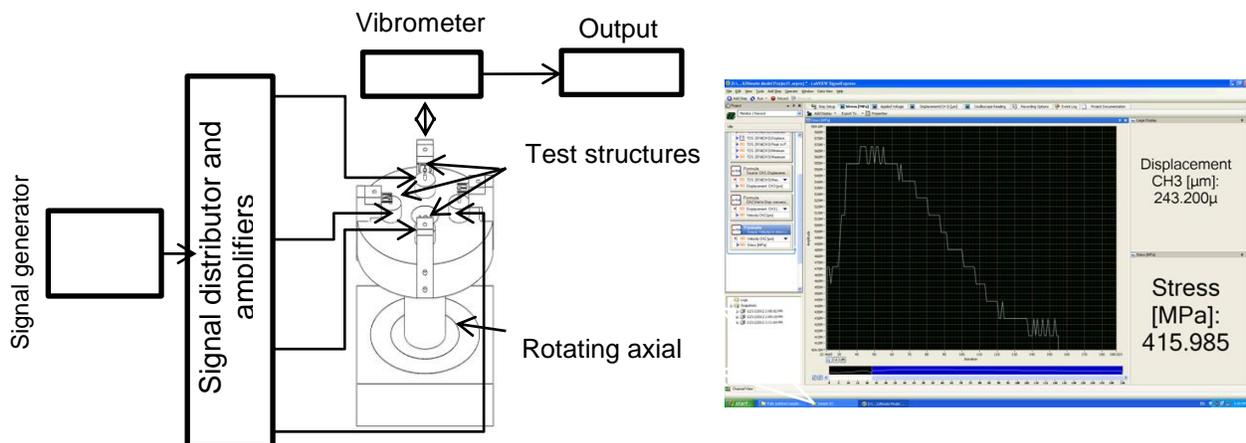
Fig. 1(a): Electromagnetic excitation setup for fatigue test (b). Stress drop during crack development
