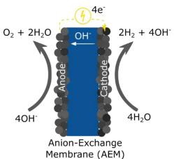
trolysis due to its efficiency, long-term stability and operation at high current densities. While PEM electrolyzers are commercially available, their costs are still high due to the acidic environment, fluorine-based membranes and noble metal catalysts. Therefore anion-exchange membrane (AEM) based electrolyzers have attracted attention, since they combine the advantageous properties of PEMWEs with the promise of significant cost reduction.
