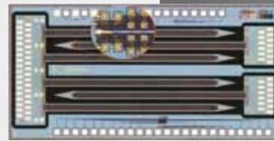
Intracortical CMOS microprobes
