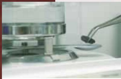
Gravimetric determination of density
