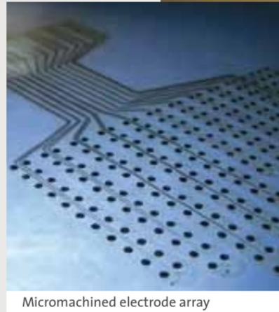
Micromachined electrode array
