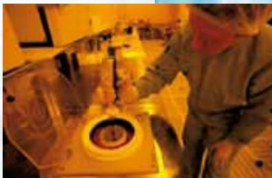
Photoresist spin coating
