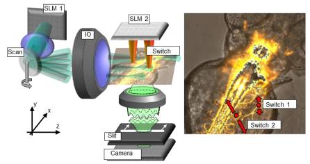
Figure: Sketch of the planned light-sheet microscope with holographically controlled illumination and optogenetic switching based on fast digital mirror devices as spatial light modulators (SLM).
